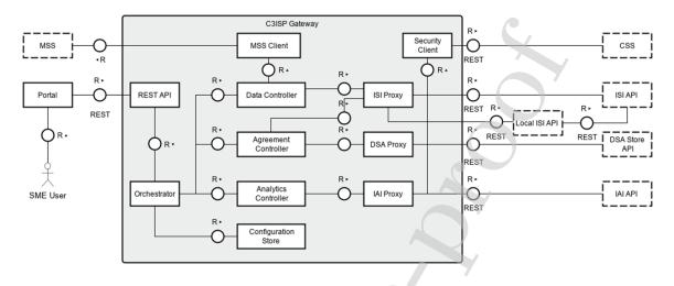
Figure 4. The C3ISP Gateway Architecture
